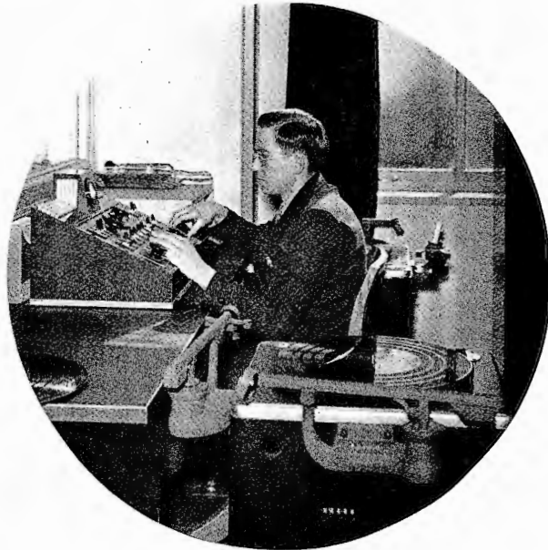
The station control room with the RCA transcription turntables conveniently located for the operator.
